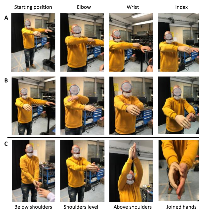
Figure 49: Coordination tests of the upper limb - A) with the prosthetic arm B) with the contralateral arm, and C) with both arms.
