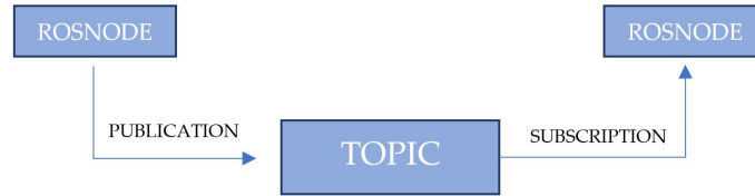
Figure 3.3: Schematic Representation of Communication between Nodes through Publisher and Subscriber
