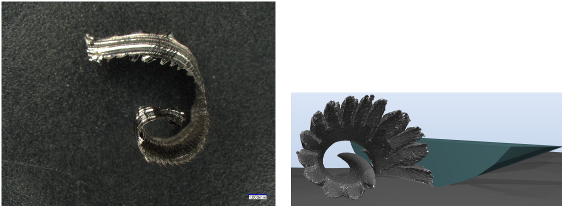
Figure 11.38: Comparison between real chip and simulated one in wet conditions, D=580\text{MPa} .
