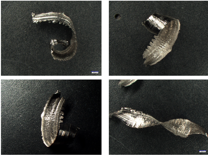
Figure 11.36: Chips formed at V_c=125 m/min, f_z=0.7 mm/rev*tooth, a_e=13 mm a_p=0.4 mm during wet machining.
