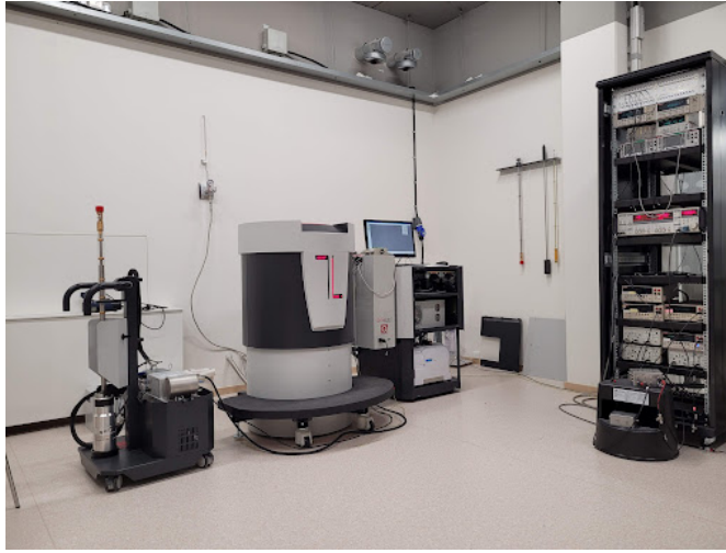
Figure 2.6: Physical Property Measurement System
