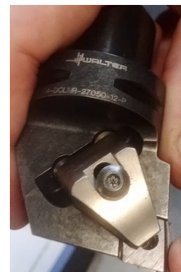
(b) Insert mounted in tool holder
