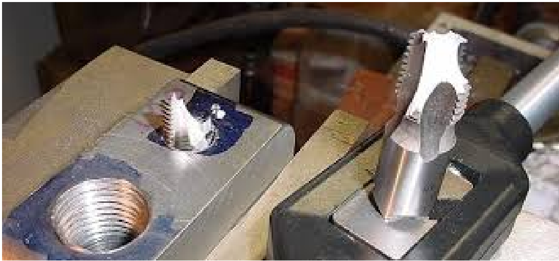
Figure 5.1: Tapping tool torsional failure
