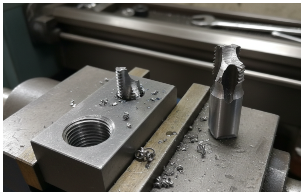
Figure 2: Tapping tool breakage
