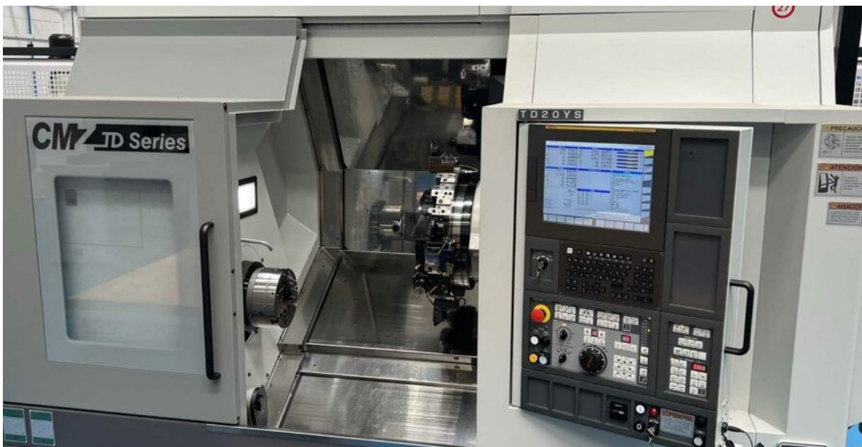
Figure 3.4: CNC lathe machine with FUNUC (i-series) control system
