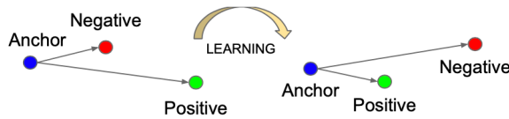
Figure 2.6: The triplet loss is a loss function which try to minimize the Euclidean distance between the positive and the anchor sample, while maximizing the one between anchor and negative samples
