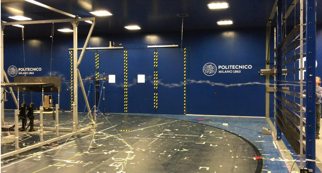
Figure 2.40. Harmonic oscillating wind velocity generated by an active turbulence generator.
