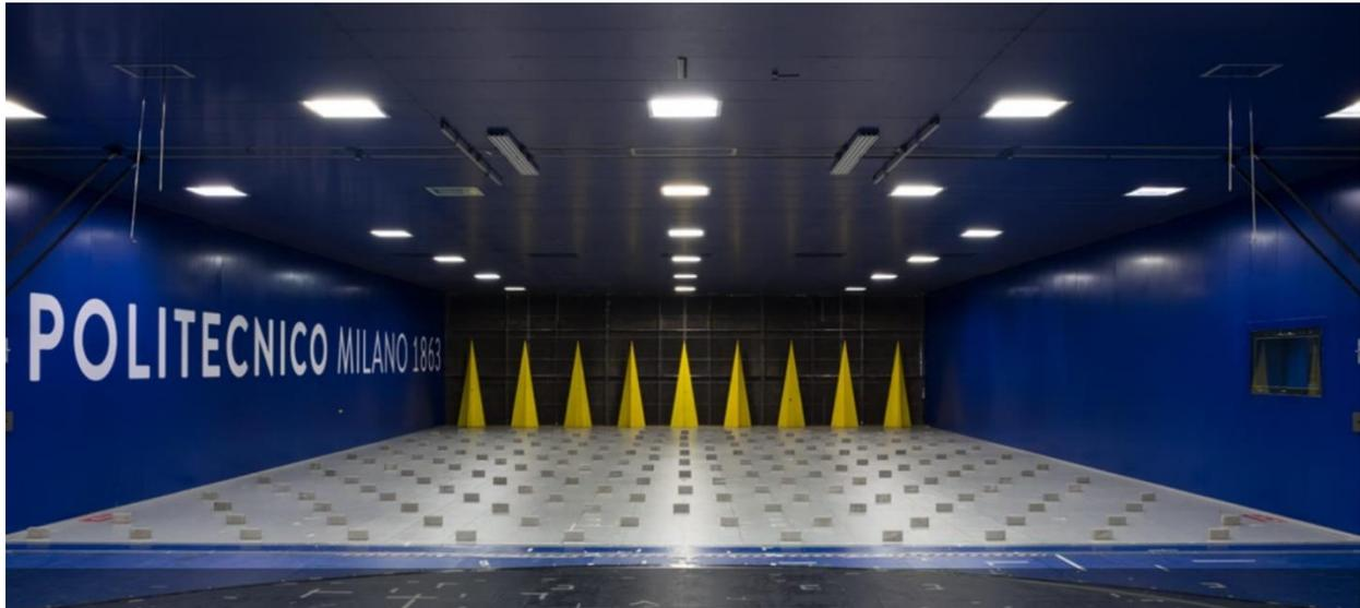
Figure 2.2. Spires and roughness elements for the simulation of the atmospheric boundary layer
