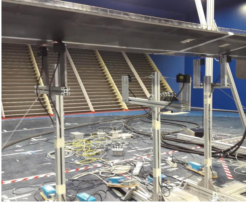
Figure 2.9. Lasers transducers below the deck sectional model.
