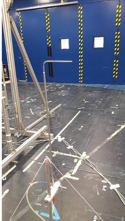
Figure 2.6. Installed Pitot tube.
