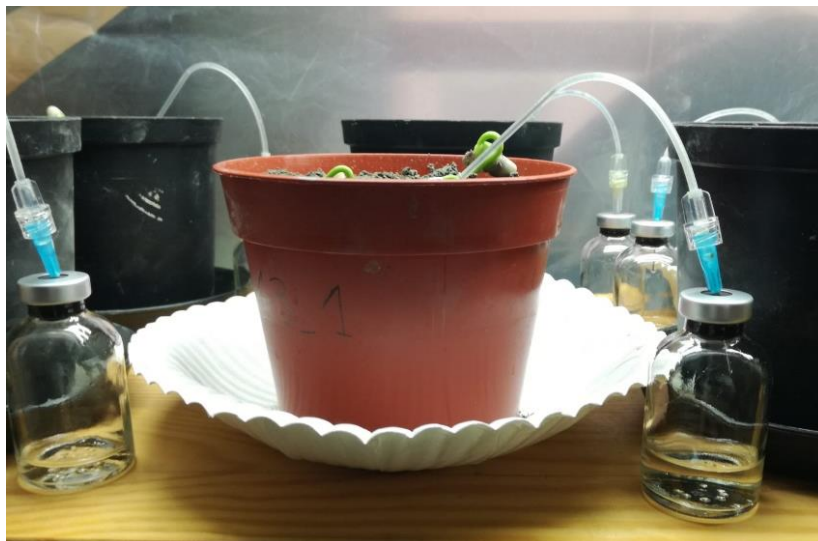
Figure 5.5. Layout used to sample the interstitial water.
