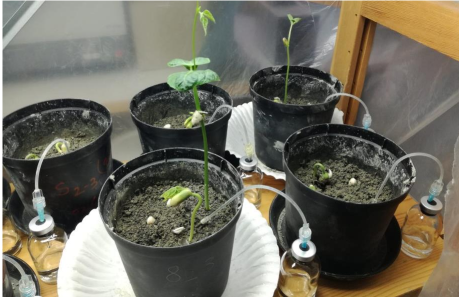
Figure 5.6. Phase of extraction of the interstitial water.
