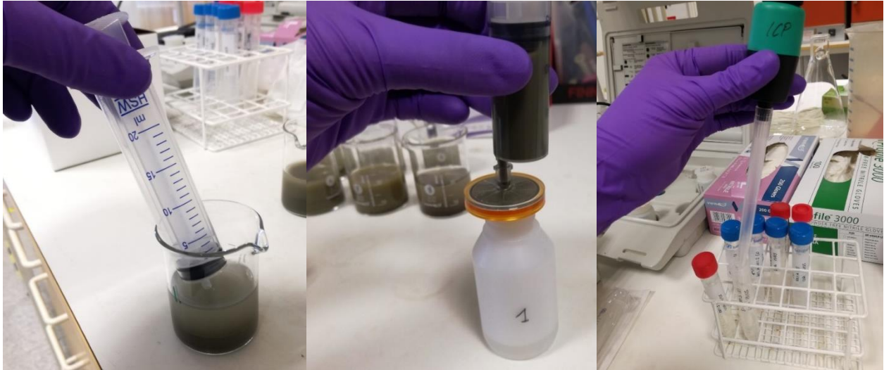
Figure 4.7. Steps to prepare samples for ICP analysis: collection, filtration, and dosage.
