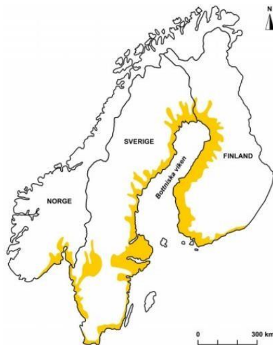
Figure 1.2. Maximum extent of the Littorina Sea about 7000 years ago and thus where sulphide soil can occur (Boman, 2010).
