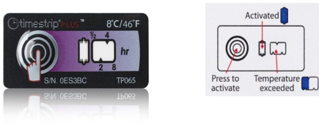
Figure 6.4: Functioning of the Timestrip time-temperature indicator (Source: Company B website)
