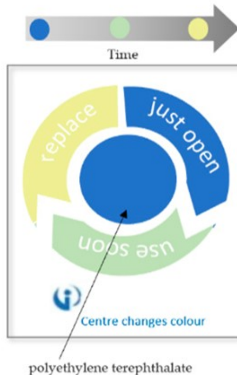
Figure 2.11: Commercial example of freshness indicator (Source: Beshai et al., 2020)
