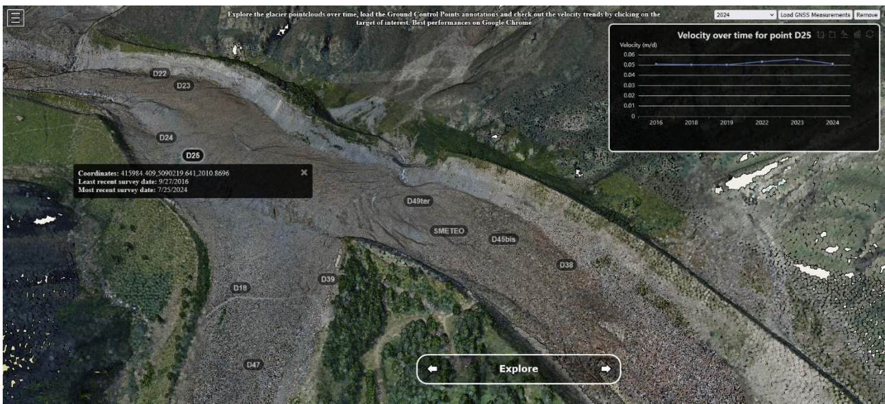
Figure 38. Example of a graphical visualisation of the velocity time series of a user-selected target measured along the glacier. The real-time connection to the geodatabase allows the query of targets measured on a given survey. The pop-up windows show additional details on each point as well as their calculated velocity trends (from Gaspari et al., 2025a).
