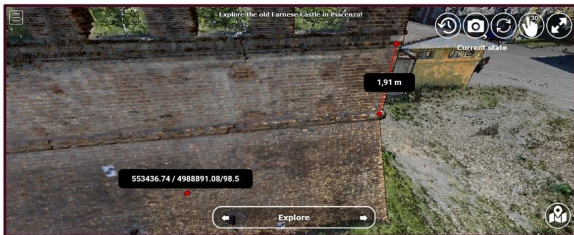
Figure 24. The distances measured on features visible on the oriented images are connected to the point clouds of the site inserted in the 3D scene. This is possible thanks to the Potree native functionalities position the drone images using their camera calibration information as well as the orientation parameters computed during the photogrammetric reconstruction and point cloud generation (from Gaspari et al., 2024a).
