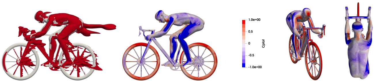
Figure 20: Total pressure coefficient on cyclist and bicycle surfaces, and isosurfaces for C_{p_{tot}} = 0
