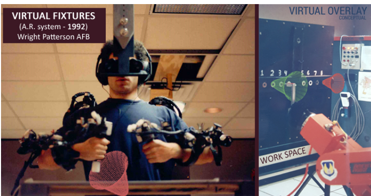
Figure 3.7: Louis Rosenberg "Virtual Fixtures", allowing computer assisted movements, 1992
