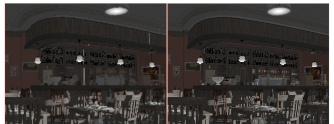
Figure 4: Difference between a 512p (left) and a 1920p (right) cube map in the "Amazon Lumberyard Bistro" scene (Open Research Content Archive).
