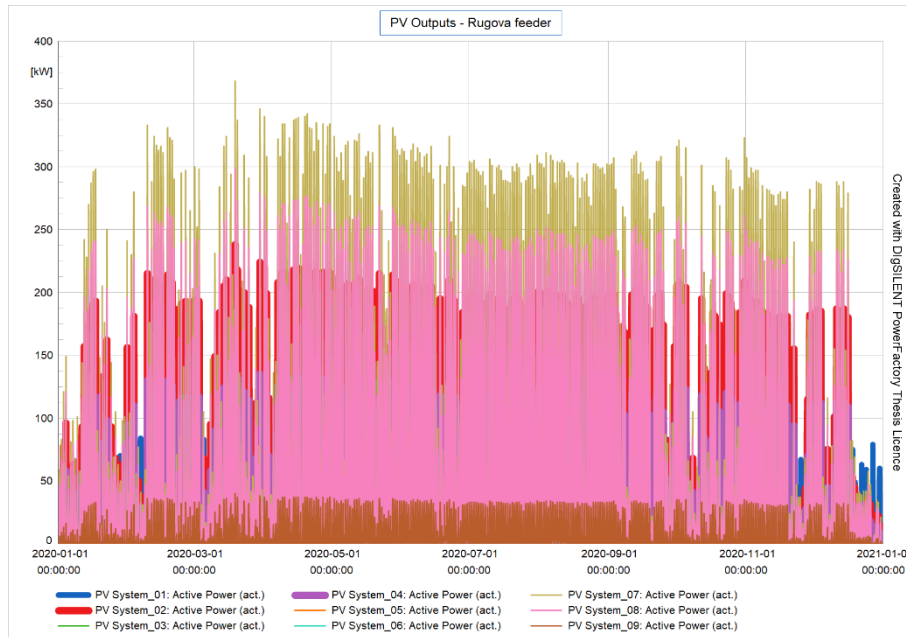
Figure 70. PV Outputs Rugova feeder (first year) [kW].
