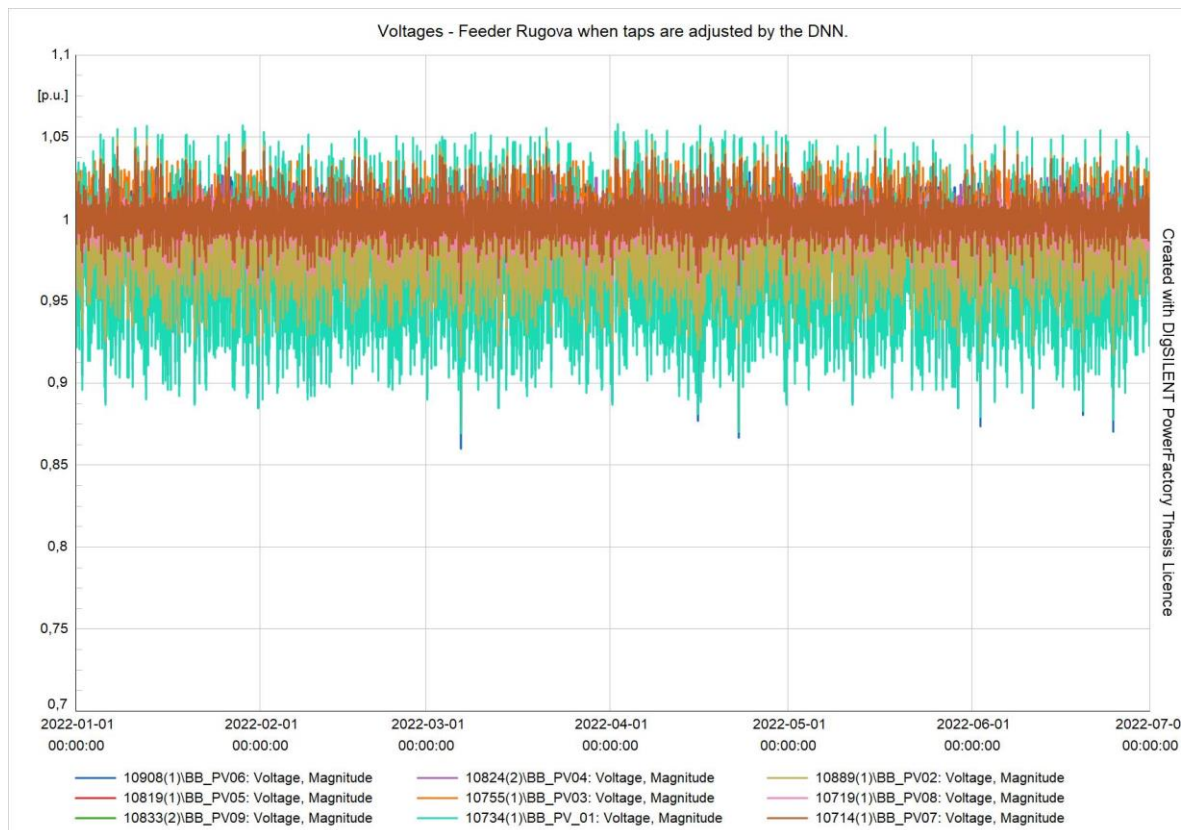
Figure 86. Voltages of Rugova feeder when taps are controlled by the DNN model [p.u.].
