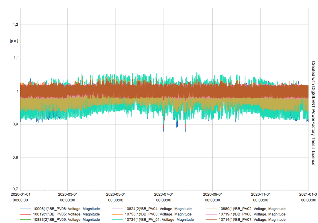
Figure 82. Voltages of Rugova when combining E-OLTCs and LVRs (first year) [p.u].
