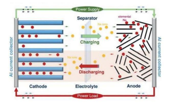
Sodium ion batteries usually take NaxMO2 as the positive electrode material and hard carbon as the negative electrode material. The reaction formula of electrode and battery can be expressed as:
