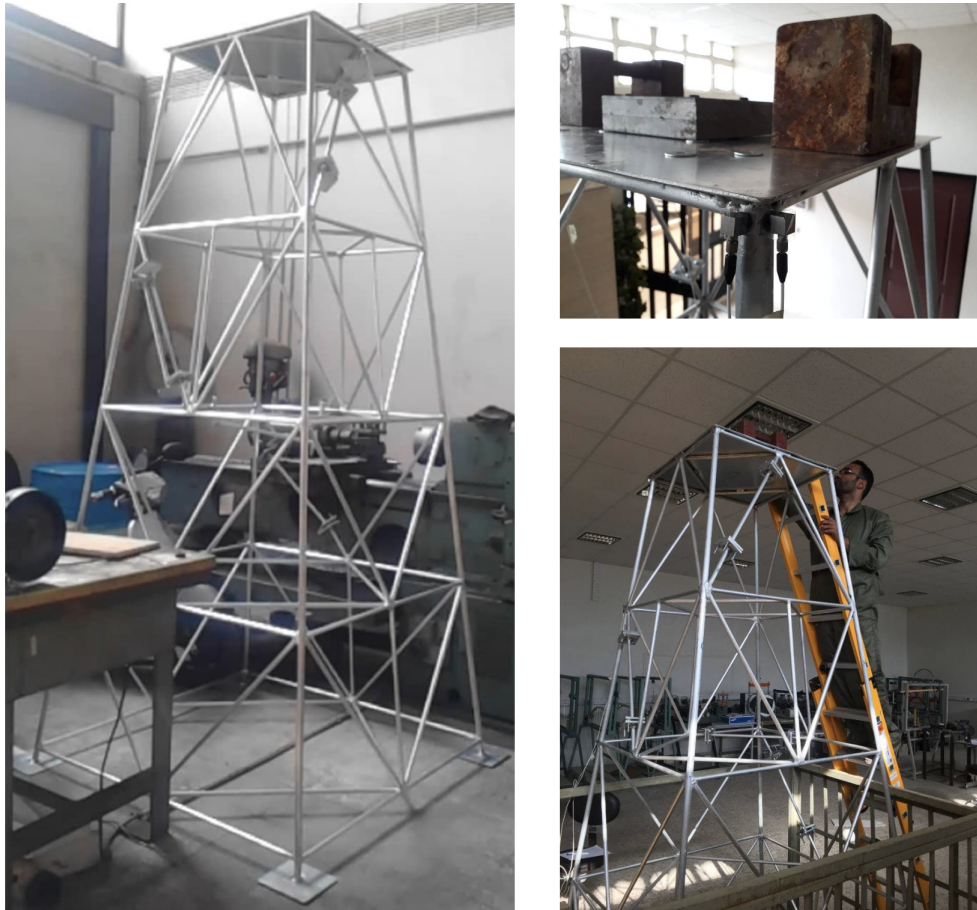
Figure 6.45: The overall view of the experimental offshore jacket platform.
