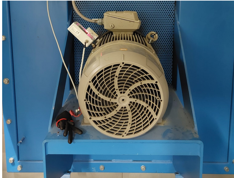
Figure 14: Sensor mounted on a fan
