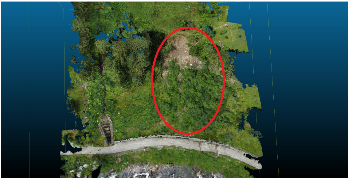
Figure 6.8: Known landslide 3D reconstruction from UAV survey
