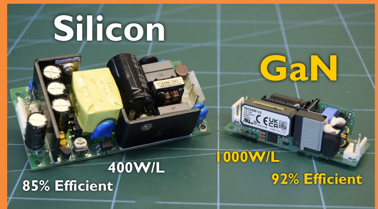
Size and power density comparison of GaN based power adapters and traditional Silicon based ones
