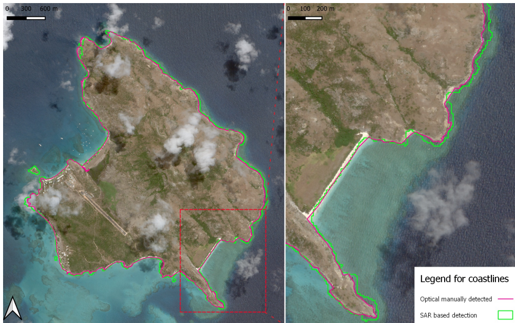
Figure 4.1: The SAR based detected coastline (in green) extracted with the process explained in Section 3.2.4 is compared to the manually digitized coastline (in green) based on the optical imagery Planet SkySat (0.8 m pixel spacing), by ©Planet Labs Inc. On the right there is an enlarged view to appreciate finer details.
