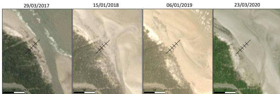
Figure 4.15: The optical acquisitions operated by ©Planet Labs Inc. Each acquisition shows the state of the coast for the area in each year, but tidal level could be different for each square. However, it is possible to appreciate the regression of the vegetated area. The black transect with the gridded bar is the same one that was on Figure 4.14, so that a comparison with the SAR analysis is possible.
