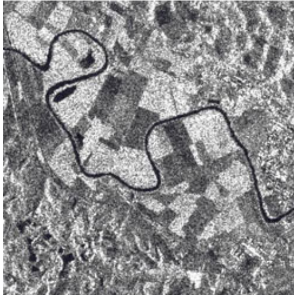
Figure 2.3: An example of speckle: the SAR scene was acquired on 21/4/1994 over Tiber Valley. It shows some agricultural fields, note the intensity variation in the homogeneous patches.
