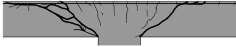
Figure 1.3: Punching shear failure mechanism
