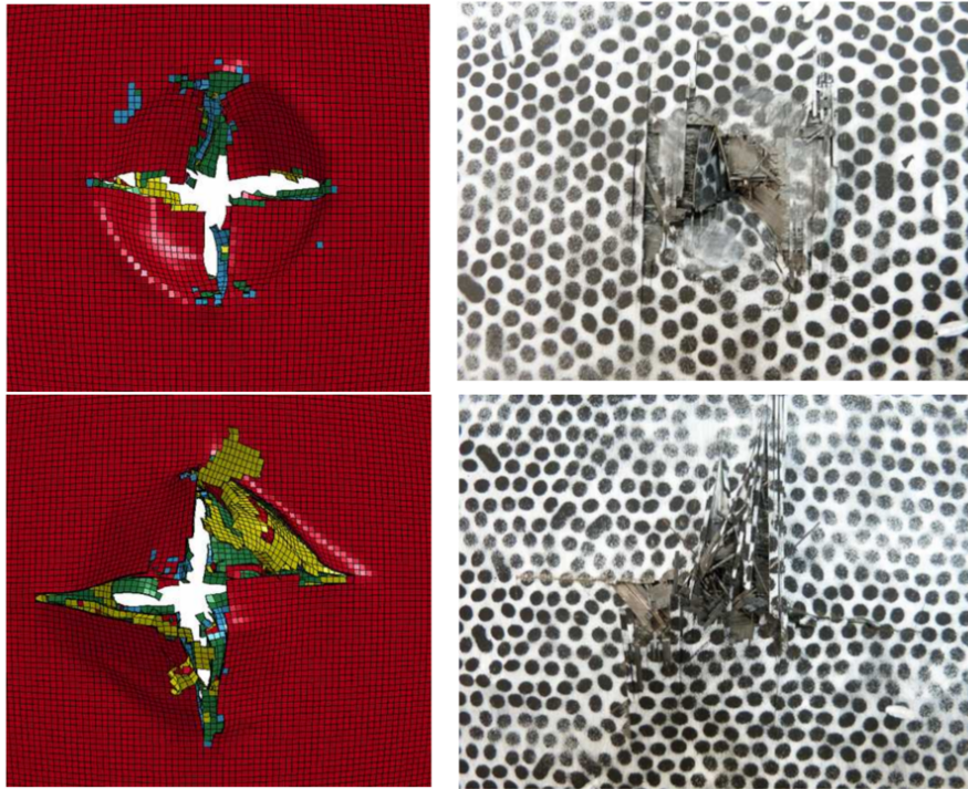
Figure 6.14: FEM vs Test fracture pattern
