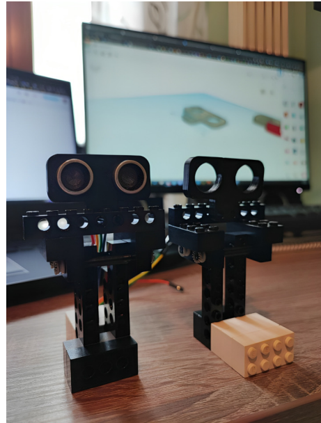
(b) Lego mount with ultrasound sensor.
