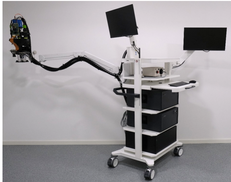
Figure 5.3: Multispectral optical imaging in real-time for surgery developed in the iCube laboratory by S. Segaud
