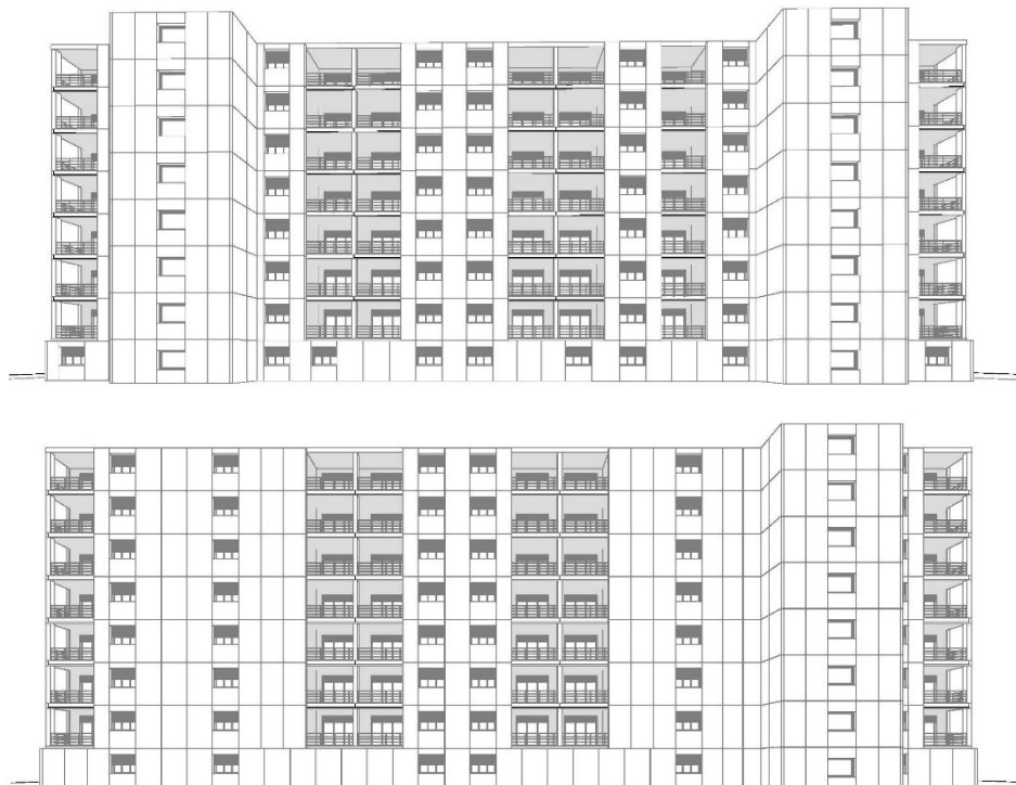
Figure 5.23_ SOUTH - EASEE panelization on the initial case study (above) VS the new model (bottom)
