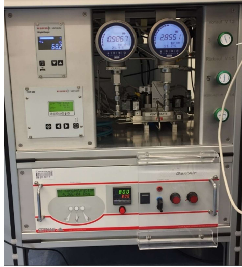
Figure 2.14: Gen'Air oxygen gauge and detector, together with the vacuum turbopump controls, its relative manometers, the valve-control plate (ventilplatte) and the manual inlet-outlet valves.
