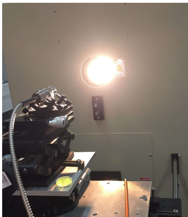
Figure 2.18: Low temperature pyrometer during calibration against the graphite blackbody furnace available at JRC
