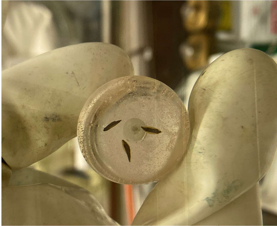
Figure 3.19: Samples after polishing embedded in a silicon matrix.
