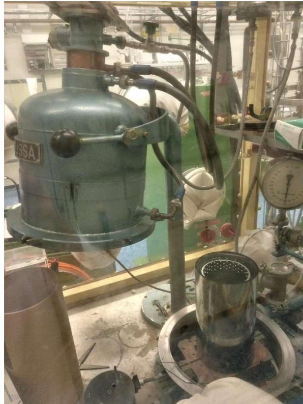
Figure 2.2: Degussa VSL 10/18-Molybdenum cold wall furnace in the Pu line at JRC Karlsruhe.
