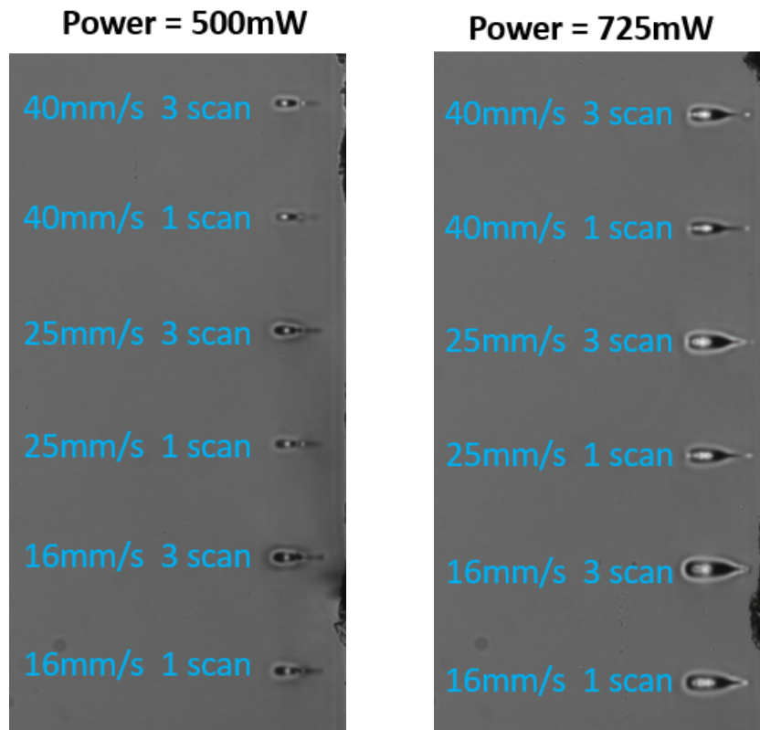
Figure 4.3: Microscope images of two groups of waveguides. The images are taken with the same magnification. The waveguides were fabricated with different powers, writing velocities and number of scans.
