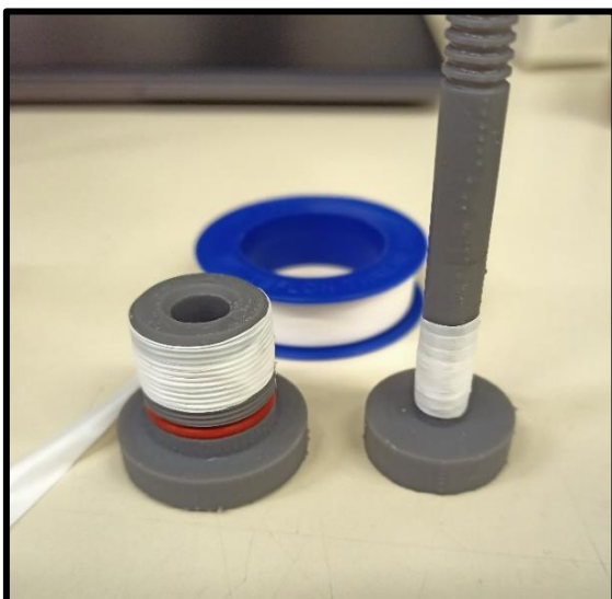
Figure 4.12 Image of the Fixing screw and Inlet axis coated with PTFE
