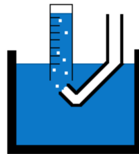
Figure 5: Small graduated cylinder submerged in a water bath is utilized to measure tidal volume over a specified number of breaths.
