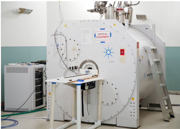
Figure 1: 9.4 Tesla preclinical MRI system within the UIC RRC Preclinical Imaging Core.
