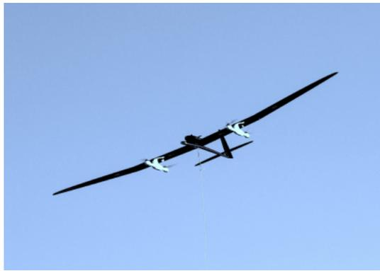
Figure 2.1: 5 kW prototype of Kitemill AS
