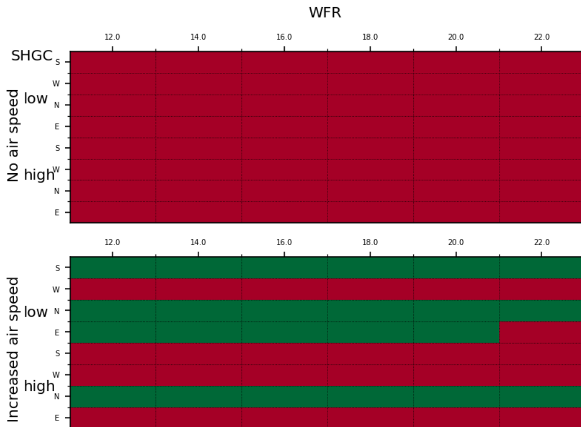
Figure 48 – TM52 compliance for all the combinations in the case of Milan with the base-case configuration and room on the middle floor and middle position
