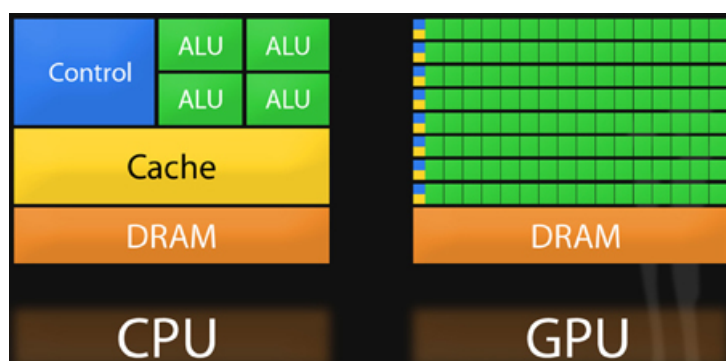
Figure 2.1: An architectural comparison between CPUs and GPUs. [12]
