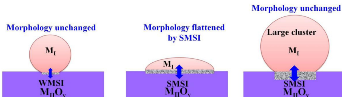
Figure 4.12: Geometric effect induced by weak or strong metal-support interaction [34].
