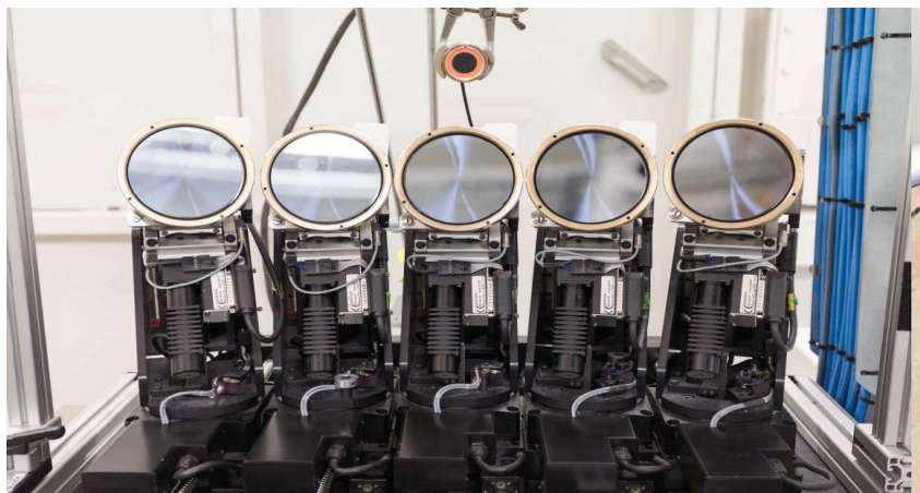
Figure 2.13: Five-analyzer crystals in experimental hutch EH2 at ID26 [18].
