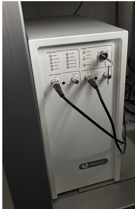
Figure A.2: LIBS excitation laser integrated in the CORALIS system.
