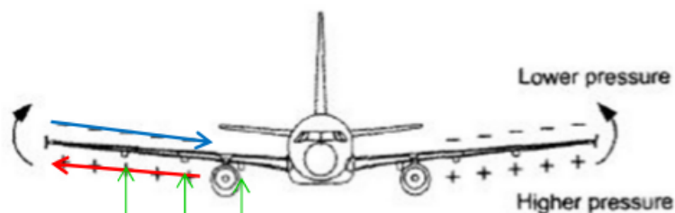
Figure 4.1. Sketch representing the difference in pressure between the two sides of an airplane wings
