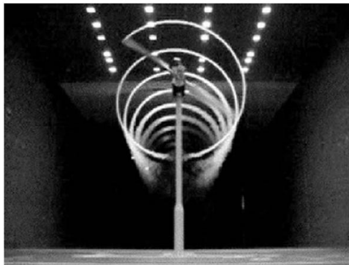
Figure 4.4. A visualization of the tip vortices characterizing a wind turbine
