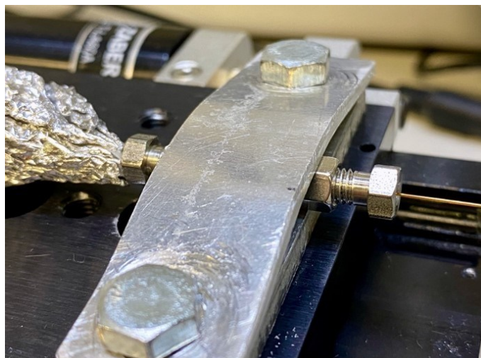
Figure 2. 22 – Connection between micro-GC line and capillary
