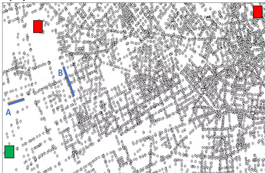
Figure S2. Representation of the urban area in which pipes A and B were renovated through relining with epoxy resins for which to assess the potential release of BPA. The DWTP feeding the renovated pipelines is reported as a green square. The DWTPs serving adjacent areas of the DWDN are reported as red squares.
