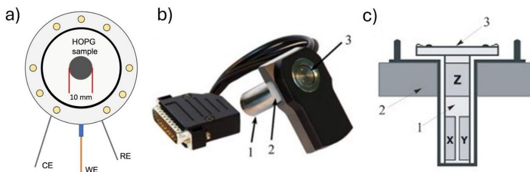
Figure 2.21: a) Electrochemical cell. b) photo of the scanner AFM, 1) scanner protection; 2) points where the screw act in order to move the scanner along the x direction; 3) scanner magnetic disk. c) schematic representation of the scanner: 1) piezoelectric that controls the movements in the 3 directions; 2) support; 3) scanner magnetic disk [108,109].
