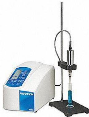
Figure 20: Sonicator. The microprobe is inserted in the tube to produce cavitation
