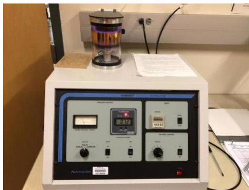
Figure 15: Hummer 8.0 Sputter System used to gold coating on the samples
