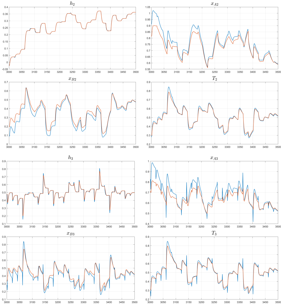
Figure 3.6: Comparison between the simulated output (—) and the REN model output (—), under high-frequency input signals.
