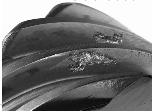
Figure 1.3.1: Pitting on the Flank Surface [21]
