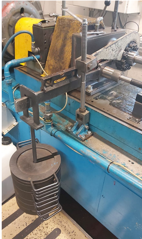
Figure 6.2.7: The Calibration Setup Installed on the FZG Hypoid Test Rig
