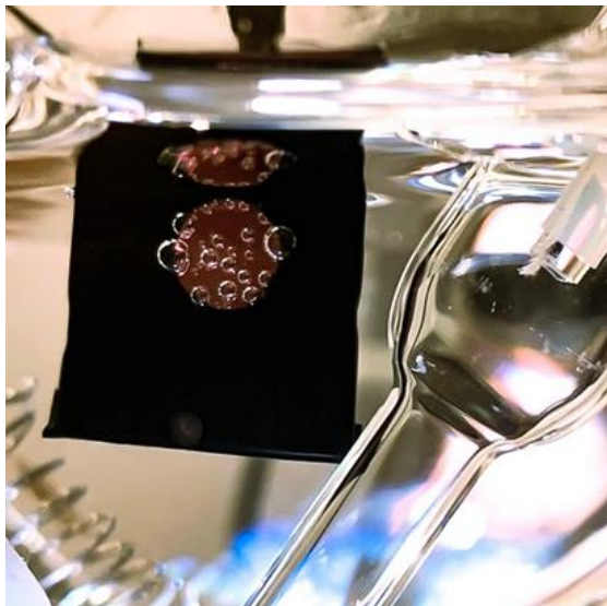
Figure 36: Picture of a HPC during operation. On its surface, H 2 bubbles can be seen.
