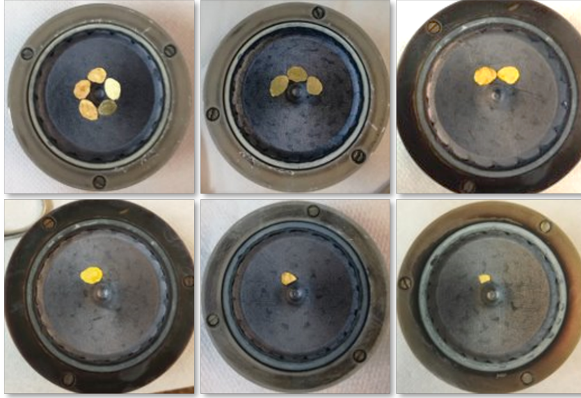
Figure 4.1: Pictures of targets employed for Au-TiO 2 co-depositions. The number of Au plates varies from 1/4 to 5.
