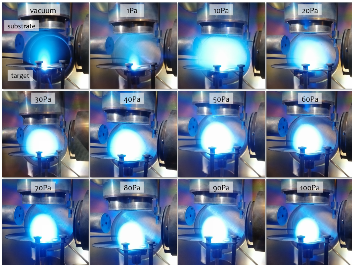
Figure 3.4: Pictures of PLD plasma plume during depositions performed by means of UV (248 nm) laser by varying background pressure from vacuum to 100 Pa ( N_2 ). It is clear how pressure affects plasma plume confinement and, as a consequence, deposition regime. Pictures taken at CNMS.
