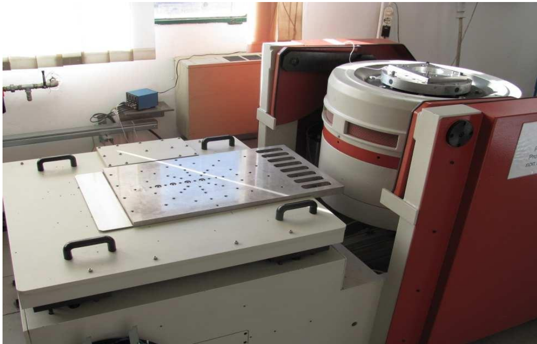
Figure 22: Electromechanical Shaker setup
