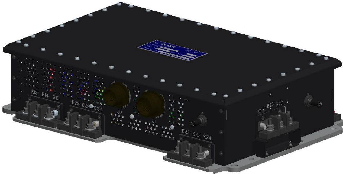
Figure 3: 3D view of AC PDP 1.
