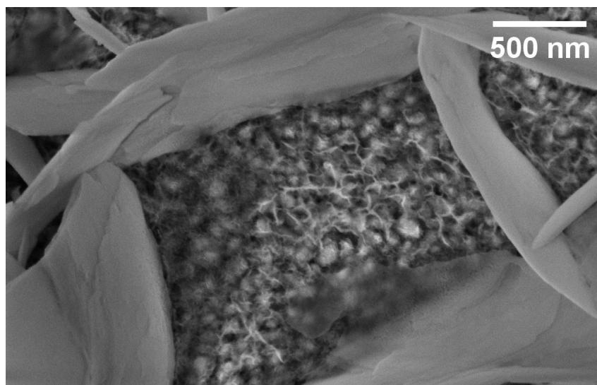
Figure 5.13: SEM image of the sample deposited at 100 Pa of oxygen and annealed at 500°C for 2 h after all the electrochemical tests. The ZHS flakes are visible.
