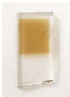
Figure 5.2: ZMO deposited in 50 Pa of oxygen and annealed at 500°C for 2 h on FTO-coated glass.
