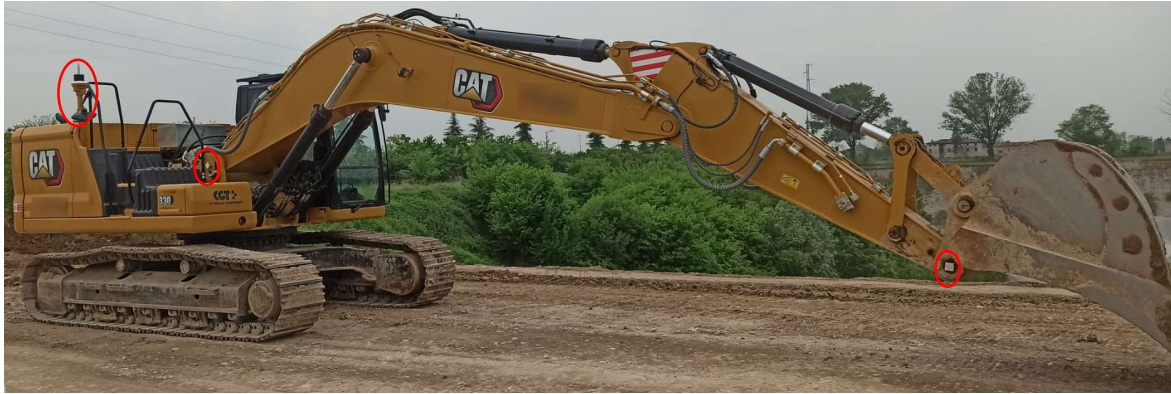
Figure 59 Target positioning (GNSS receiver, boom and bucket hinges)
