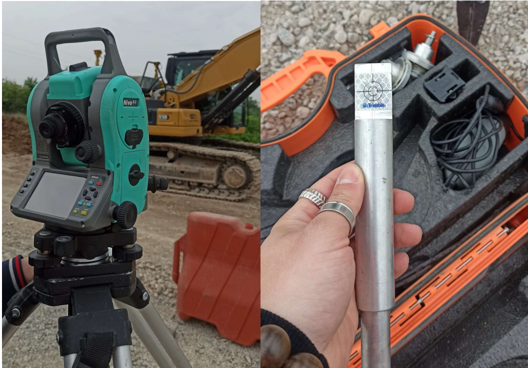
Figure 57 Total station and Targets
