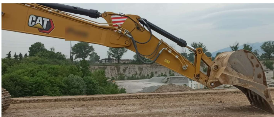
Figure 58 Correct Positioning of the Boom, stick and bucket
