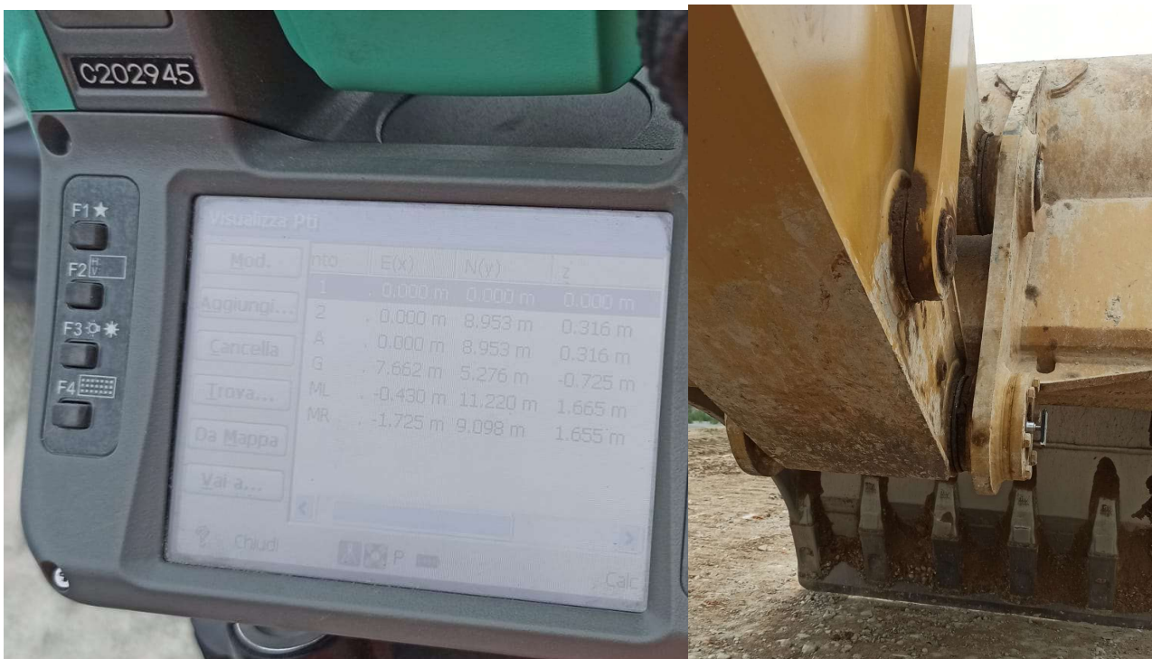
Figure 60 Point list on TS (left) and Target position offset on bucket hinge (right)
