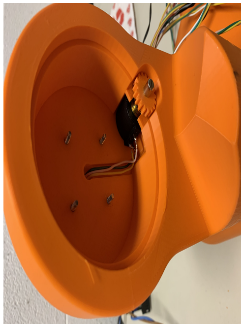
Figure 3.28: J2 potentiometer mounting system
