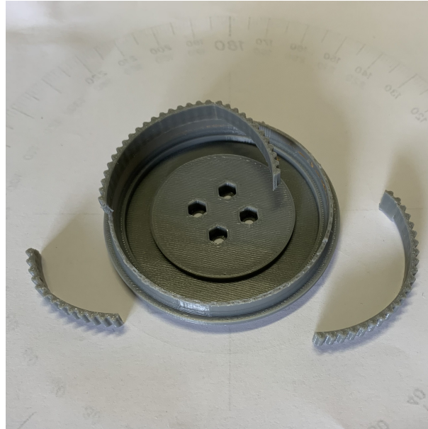
Figure 7.1: Broken flexible spline
