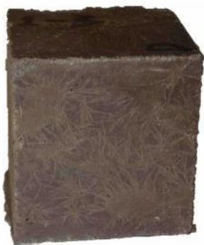
Figure 19. A simulant from Martian Concrete (Wan et al., 2016).
