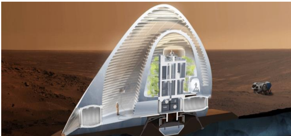
Figure 76. Sectional view through the interior revealing double wall condition (M. Morris et al., 2016b).
