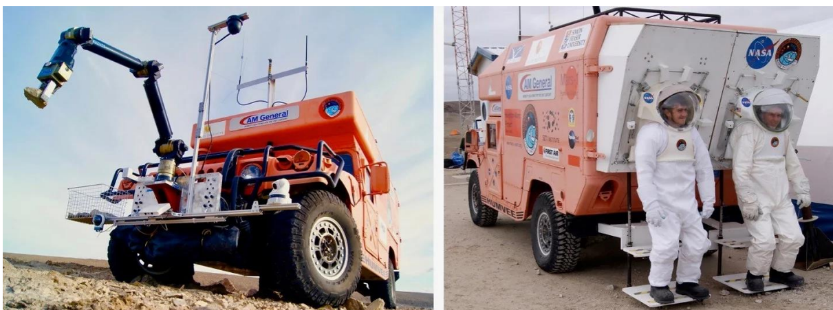
Figure 25. The construction and resource utilization explorer and spacesuit implementation (Olson et al., 2011).
