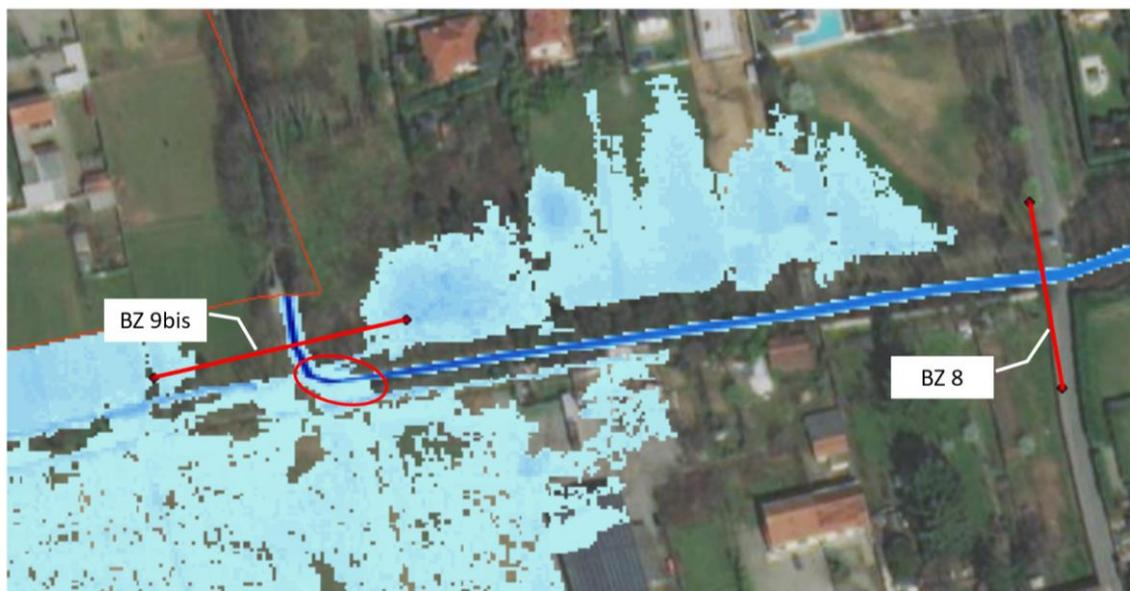
*Figure 5.16: Overflow of the Bozzente between section BZ 9 bis and BZ 8*
