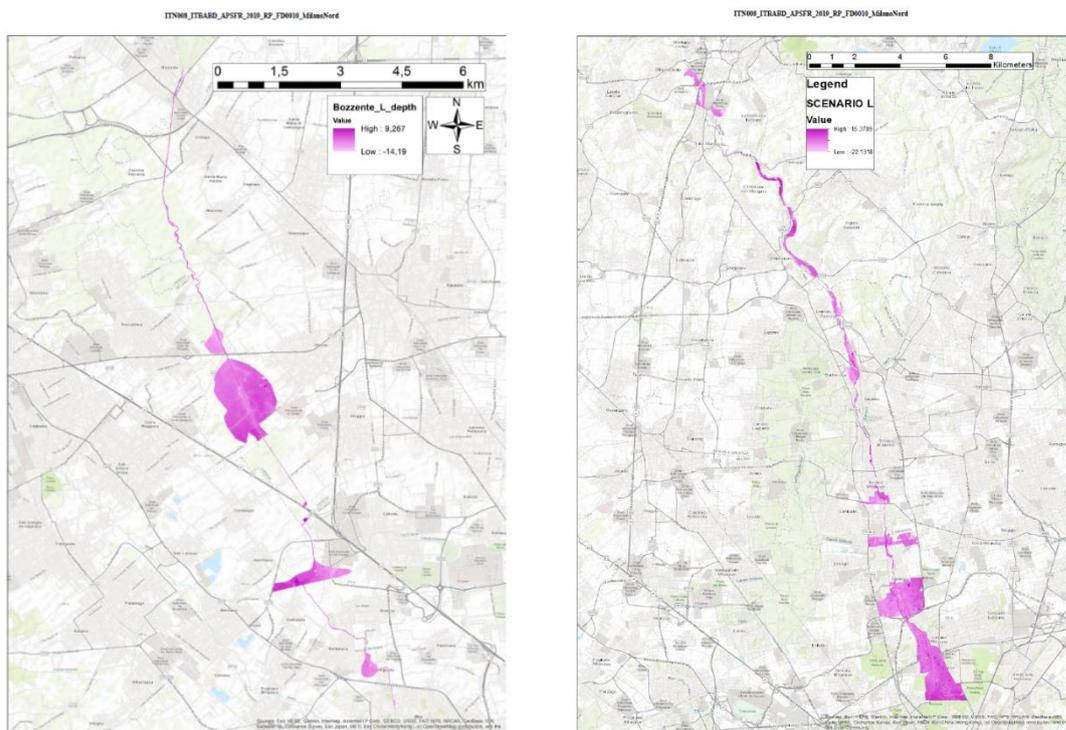
Figure 1.5: Water depth maps for Bozzente (left) and Seveso (right), 2019 version
