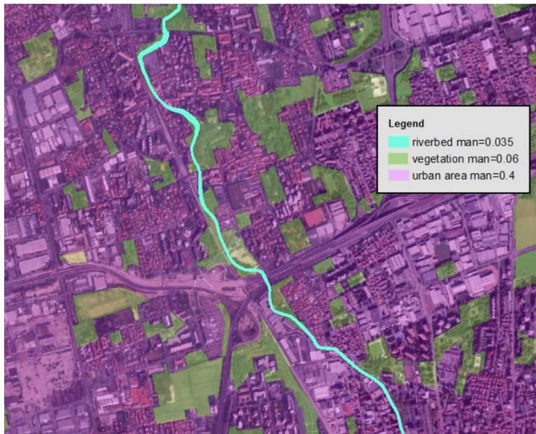
*Figure 2.3: Representation of the Manning's roughness embedded in a larger computational domain*
