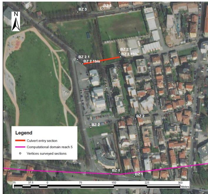
*Figure 5.12: Representation of culvert section in Bozzente River*
