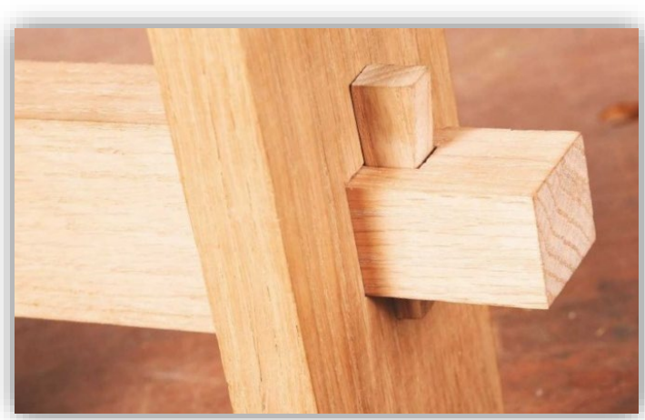
Figure 10. Mortise and tenon joint with securing pin
